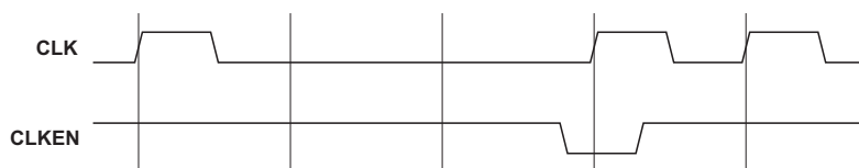
Figure 5-3 Using CLK and CLKEN for best interrupt latency
