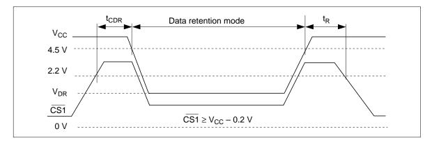
Low V<sub>CC</sub> Data Retention Timing Waveform (2) (CS2 Controlled)
