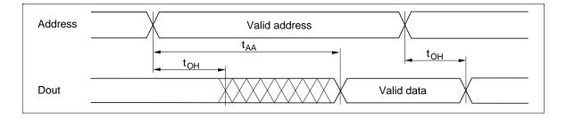
Read Timing Waveform (3)  $(\overline{WE} = V_{IH}, \overline{OE} = V_{IL})^{*3}$
