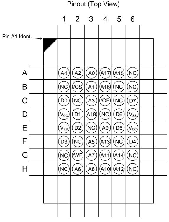
Note : Pinout shows top view, balls facing down.
