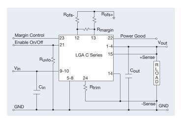
External input fusing is recommended.
