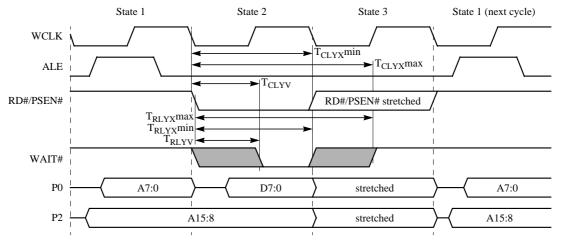
Figure 22. Real-time Synchronous Wait State: Code Fetch/Data Read
