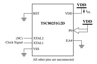
Figure 14.  $I_{DL}$  Test Condition, Idle Mode
