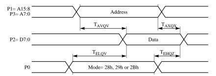
Figure 32. EPROM Verifying Waveforms
