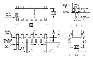
Figure 36. Plastic Dual In Line
