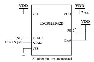
Figure 13. I<sub>DD</sub> Test Condition, Active Mode
