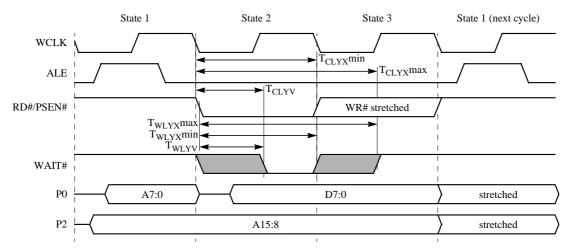
Figure 23. Real-time Synchronous Wait State: Data Write
