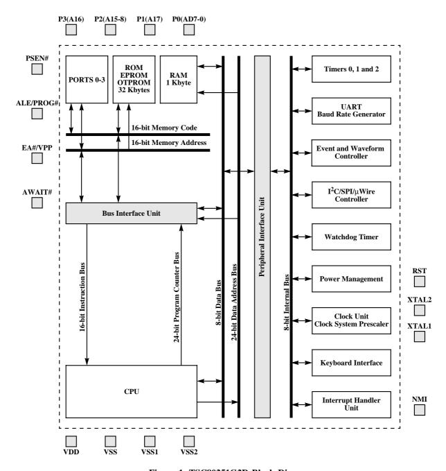
Figure 1. TSC80251G2D Block Diagram
