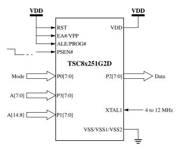
Figure 10. Setup for Verifying
