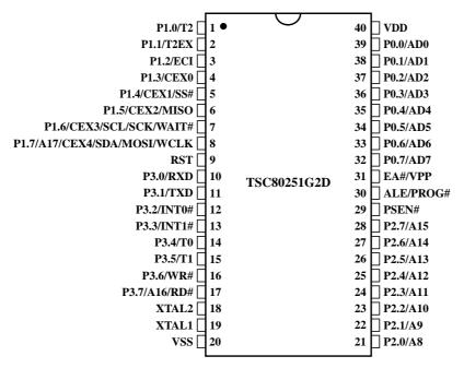
Figure 2. TSC80251G2D 40-pin DIP package
