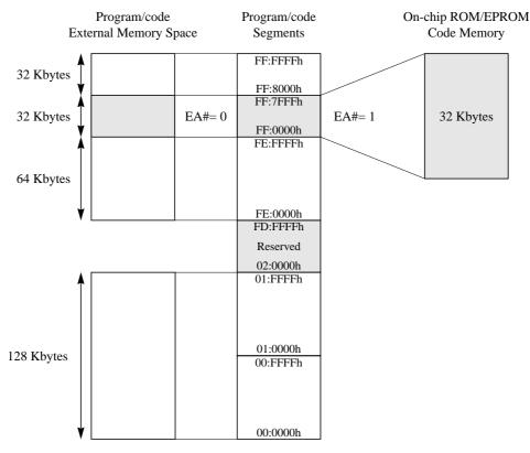
Figure 5. Program/Code Memory Mapping
