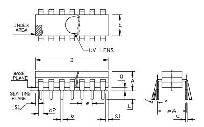
Figure 37. Ceramic Dual In Line
