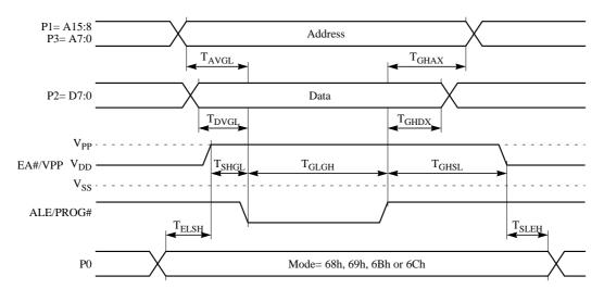
Figure 31. EPROM Programming Waveforms
