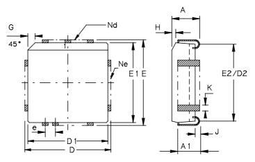
Figure 38. Plastic Lead Chip Carrier
