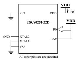
Figure 15. I<sub>PD</sub> Test Condition, Power-Down Mode
