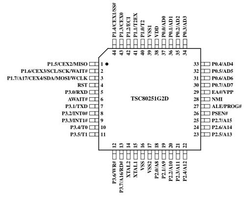
Figure 4. TSC80251G2D 44-pin VQFP Package
