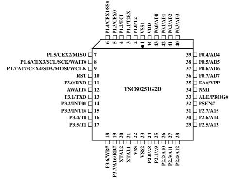
Figure 3. TSC80251G2D 44-pin PLCC Package
