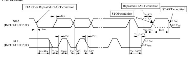
Figure 26. I<sup>2</sup>C Waveforms
