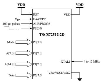
Figure 9. Setup for Programming
