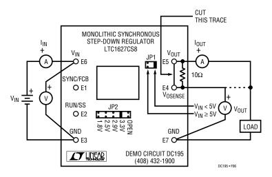
Figure 7. Remote Output Voltage Sense
