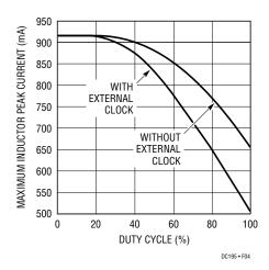
Figure 5. Maximum Inductor Peak Current Vs Duty Cycle
