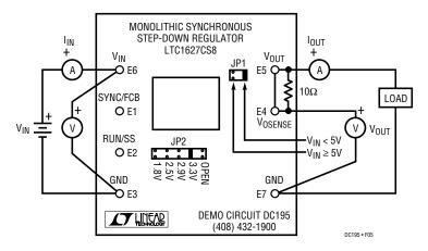
Figure 6. Proper Measurement Setup
