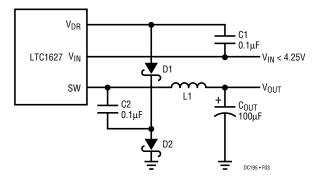
Figure 4. Using a Charge Pump to Bias VDR
