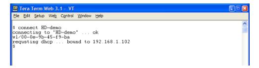
The EVK1104/1105 assigned IP address will be printed during the connection procedure (see the figure above). It should now be possible to connect to the web server using a browser on a PC that is connected to the same network.
