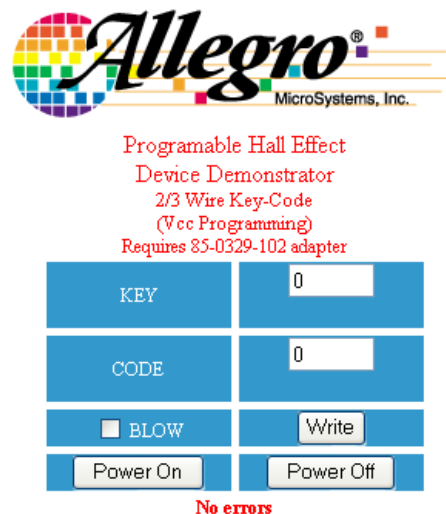
Figure 4-3 ASEK page for switch/latch programming. Reference to the “adapter” is to the optional switch/latch interface PCB.
