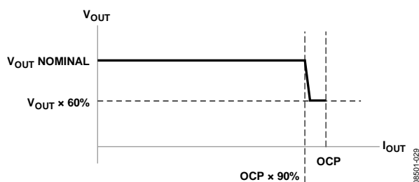
Figure 30. Constant Current Mode ( V_{OUT} vs. I_{OUT} )
