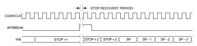
Figure 7-14. STOP Mode Recovery From Interrupt
