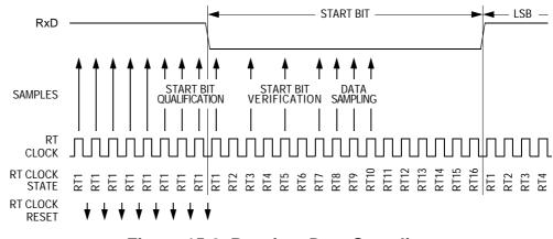
Figure 15-8. Receiver Data Sampling
