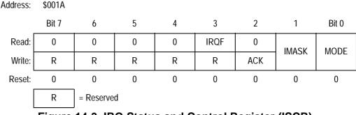
Figure 14-3. IRQ Status and Control Register (ISCR)
