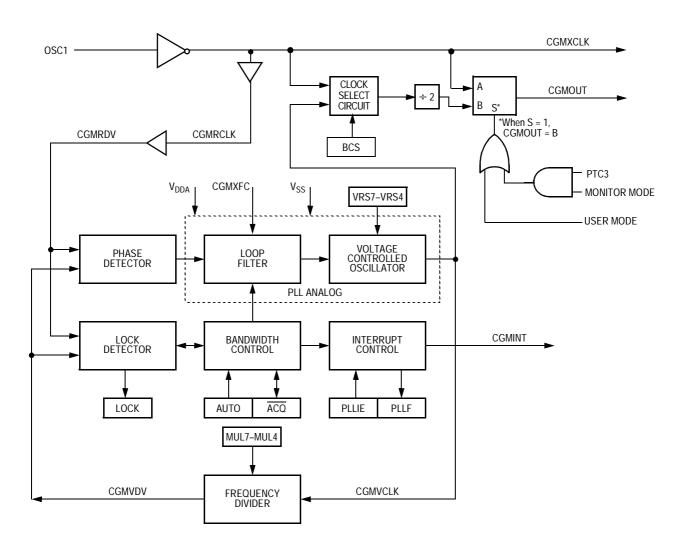
Figure 8-1. CGM Block Diagram
