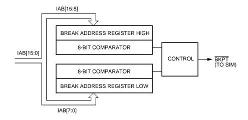
Figure 10-1. Break Module Block Diagram
