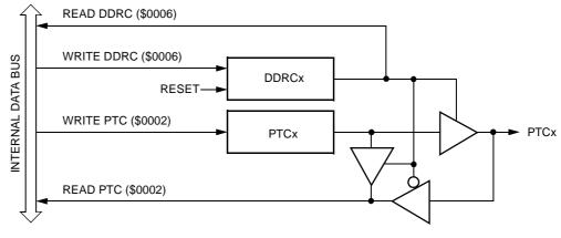
Figure 19-9. Port C I/O Circuit
