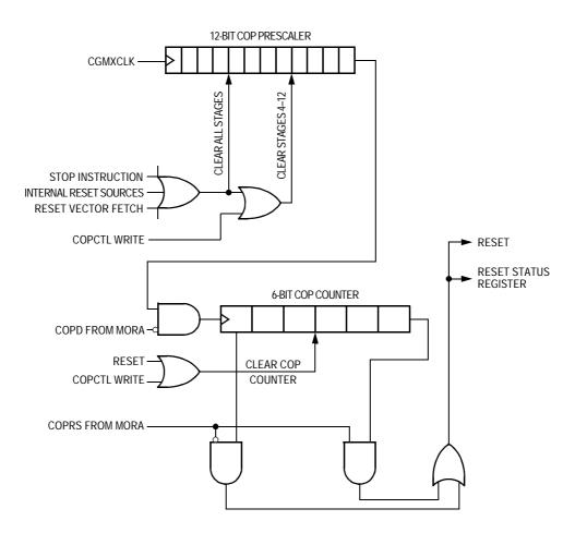
Figure 12-1. COP Block Diagram
