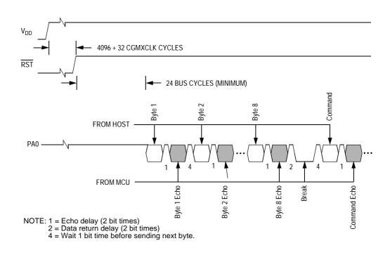
Figure 11-6. Monitor Mode Entry Timing
