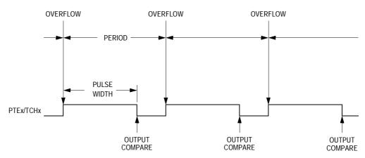
Figure 22-3. PWM Period and Pulse Width
