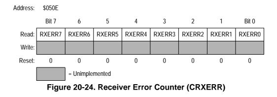
This register reflects the status of the MSCAN08 receive error counter. The register is read only.
