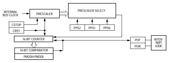
Figure 18-1. PIT Block Diagram
