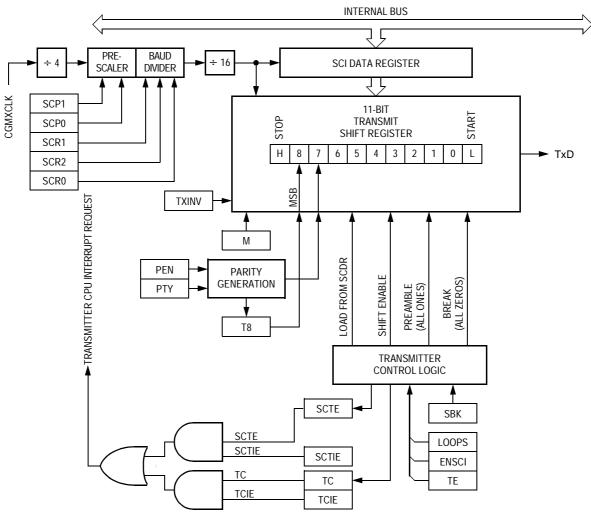
Figure 15-4. SCI Transmitter
