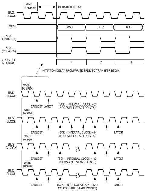
Figure 16-6. Transmission Start Delay (Master)
