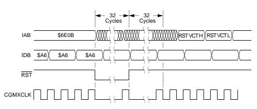
Figure 7-12. WAIT Recovery From Internal Reset
