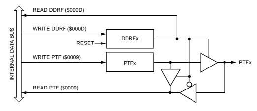
Figure 19-18. Port F I/O Circuit
