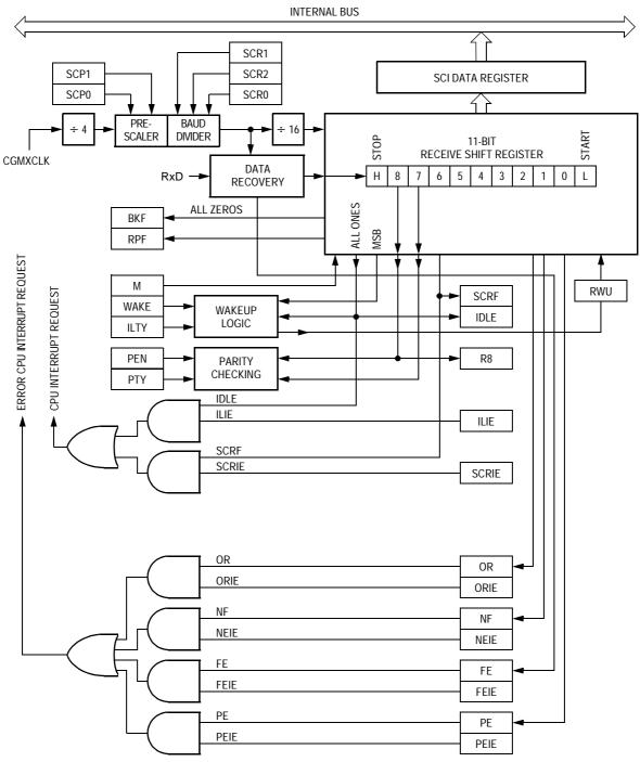
Figure 15-6. SCI Receiver Block Diagram
