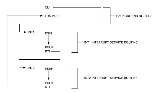
Figure 7-9. Interrupt Recognition Example
