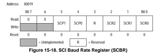
SCP1 and SCP0 — SCI Baud Rate Prescaler Bits
