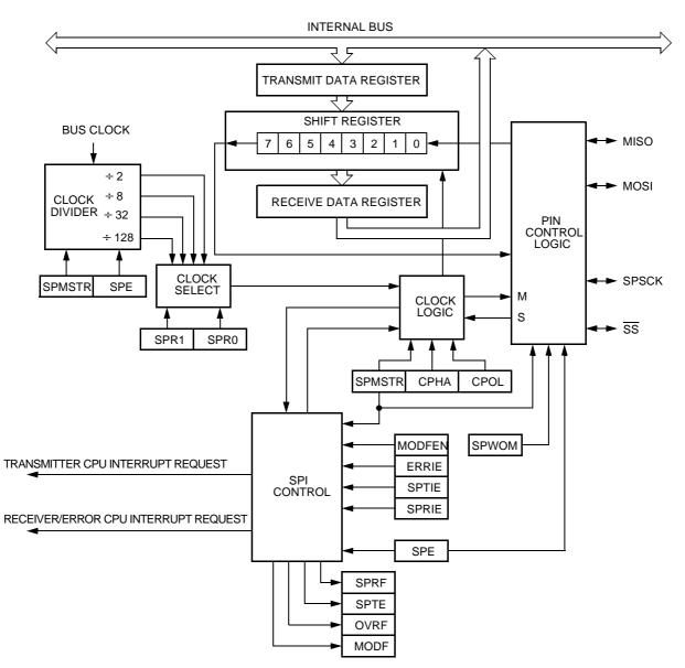
Figure 16-2. SPI Module Block Diagram
