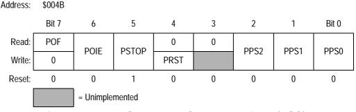
Figure 18-3. PIT Status and Control Register (PSC)
