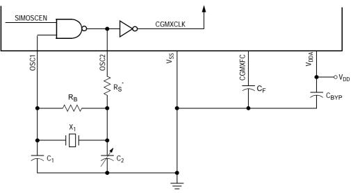
$^{\ast}\text{R}_{S}$  can be 0 (shorted) when used with higher-frequency crystals. Refer to manufacturer's data.
