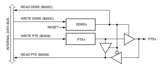
Figure 19-15. Port E I/O Circuit
