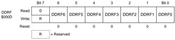
Figure 19-17. Data Direction Register F (DDRF)
