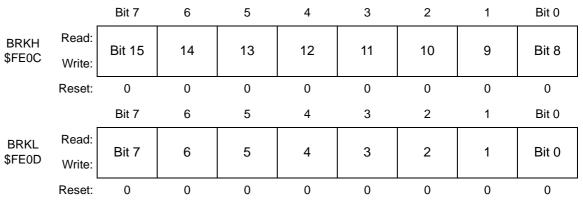
Figure 10-3. Break Address Registers (BRKH and BRKL)
