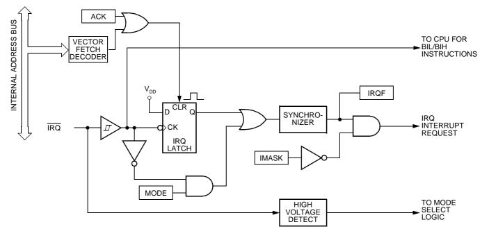
Figure 14-1. IRQ Module Block Diagram
