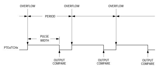
Figure 17-3. PWM Period and Pulse Width
