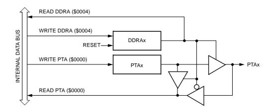
Figure 19-3. Port A I/O Circuit
