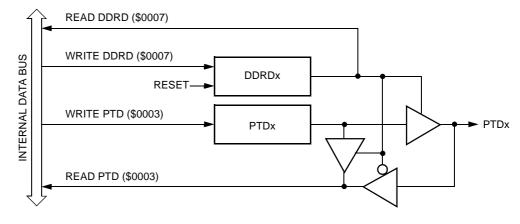
Figure 19-12. Port D I/O Circuit
