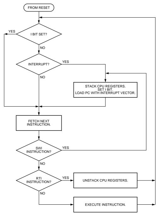
Figure 14-2. IRQ Interrupt Flowchart
