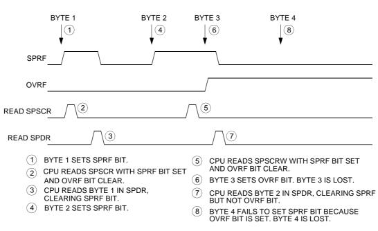
Figure 16-7. Missed Read of Overflow Condition
