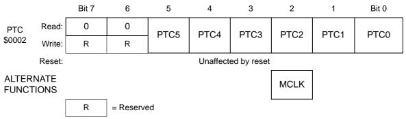
Figure 19-7. Port C Data Register (PTC)
