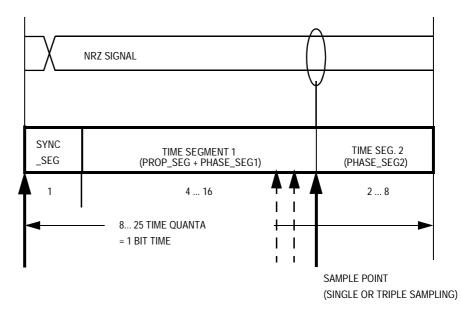
Figure 20-8. Segments Within the Bit Time
