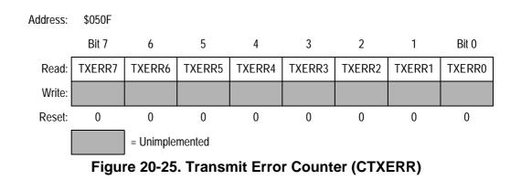
This register reflects the status of the MSCAN08 transmit error counter. The register is read only.
