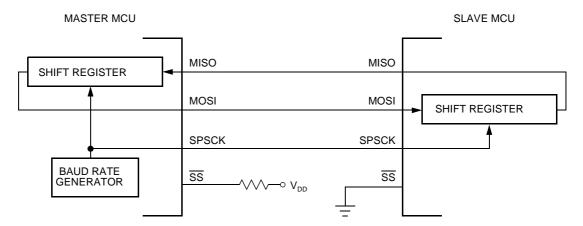
Figure 16-3. Full-duplex Master-Slave Connections
