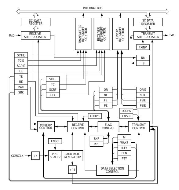
Figure 15-1. SCI Module Block Diagram
