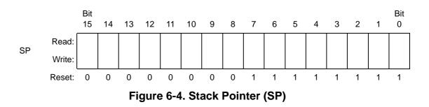
**NOTE:** The location of the stack is arbitrary and may be relocated anywhere in RAM. Moving the SP out of page zero (\$0000 to \$00FF) frees direct address (page zero) space. For correct operation, the stack pointer must point only to RAM locations.
