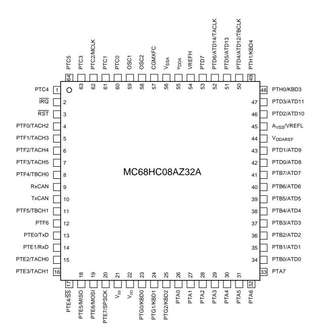
Figure 1-2. 64 QFP Pin Assignments
