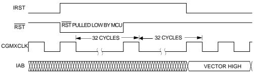
Figure 7-4. Internal Reset Timing
