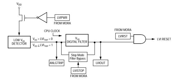
Figure 13-1. LVI Module Block Diagram
