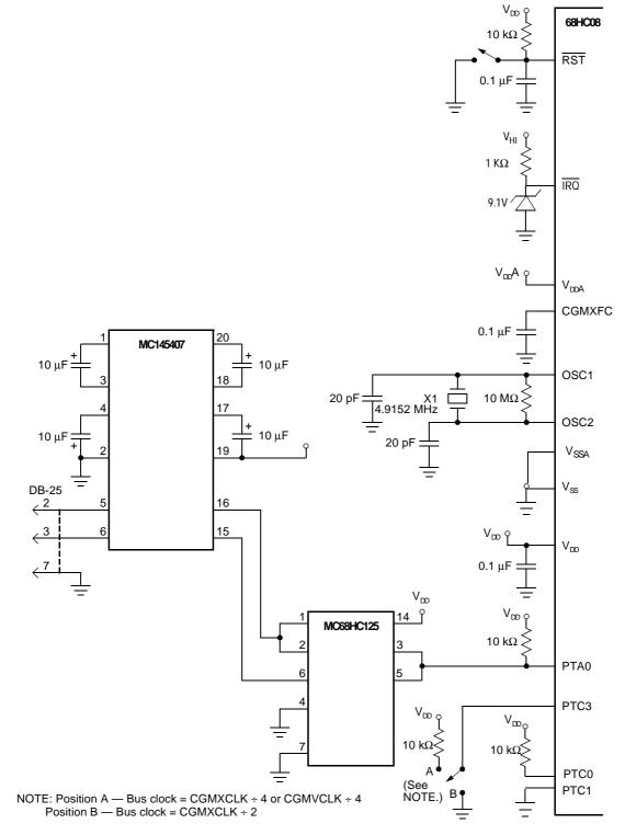
Figure 11-1. Monitor Mode Circuit
