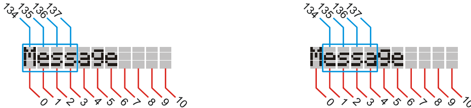
Figure 1-21: Shifting Text Through Window, Steps 3 and 4
