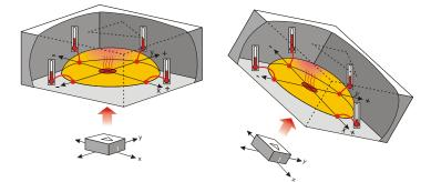
By tilting the accelerometer, the hot gas will collect closer to some of temperature sensors. By comparing the sensor temperatures, both static acceleration (gravity and tilt) and dynamic acceleration (like taking a ride in a car) can be detected. The MX2125 converts the temperature measurements into signals (pulse durations) that are easy for microcontrollers to measure and decipher.
