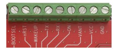
Figure 14: Terminal block (picture turned by 90° ccw)
