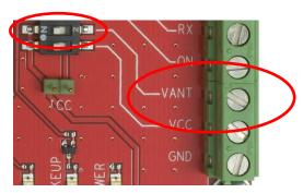
Figure 12: Antenna connector and VANT DIP switch with terminal
