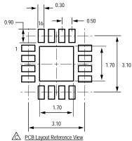
For reference only, not for tooling use (reference JEDEC MO-220WEED) Dimensions in millimeters
