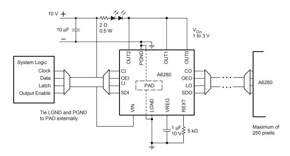
Figure 9. Application Driving High Power LED at 450 mA
