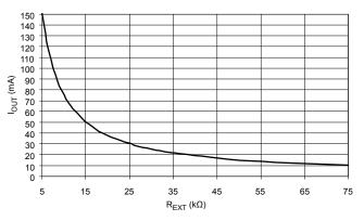
Figure 5. Output Current versus External Resistor, R<sub>EXT</sub>
