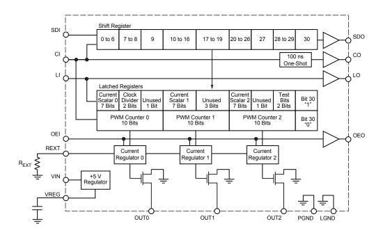
Figure 4. Functional Diagram
