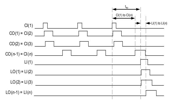
Figure 7. Signal Delay Mismatch Timing Diagram.  $t_{su}$  is the setup time for signals (CI to LI) applied to the first pixel in the chain. Note the difference in delay for CI(1) to CI(n) compared to the delay for LI(1) to LI(n). This must be compensated by increasing  $t_{su}$ .
