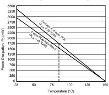
Power Dissipation versus Ambient Temperature
