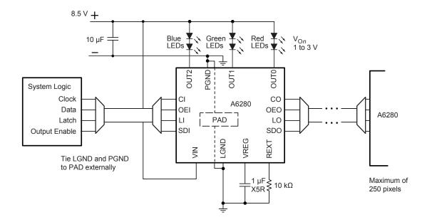
Figure 8. Application Driving 3 RGB LEDs at 75 mA Peak
