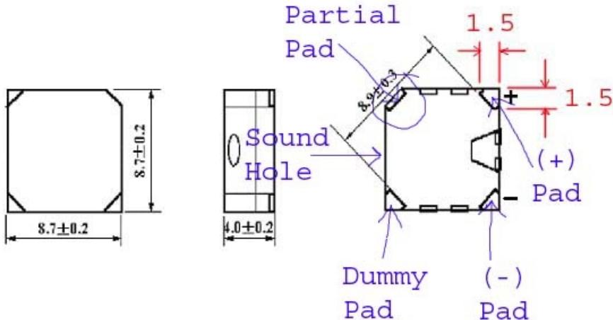
\* Dummy pad and Partial Pad are connected internally and are intended to only be used to help secure the part to the circuit board.
