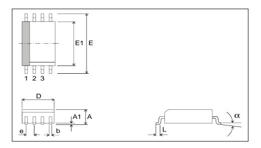
Fig. 6: SOIC8 (Small Outline Package)
