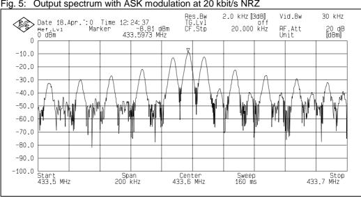
Fig. 5: Output spectrum with ASK modulation at 20 kbit/s NRZ
