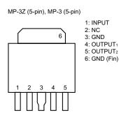
**PIN CONFIGURATION (Marking Side)**
