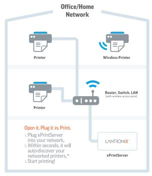
\*Each xPrintServer supports unlimited iOS devices, up-to 8 USB printers and upto 2 network printers. USB hub required to connect more than 1 USB printer.
