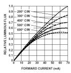
Figure 4. HPWT-xx00 Relative Luminous Flux vs. Forward Current.
