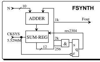
The SC-CLK is defined to be 16 times the center-frequency of the bandpass filters. For generating the FSK or MIXERfrequency, Fsynth gets divided by 16 for generation of proper DAC input signals.
