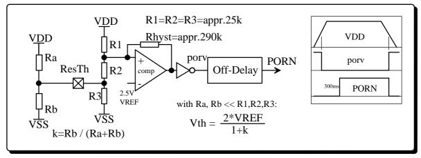
With V(ResTh) defined by external resistors much smaller than R1-3, the POR- threshold can be set in the range of 2.5V to 5.0V according to the given equation.
