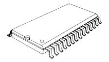
Max. Body Length Max. Body Width 7.6mm / 300mil 1.27mm / 50mil
