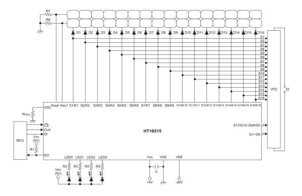
Note:  $R_{OSC}$ =82k $\Omega$  for oscillator resistor R1=1~10k $\Omega$  for external pull-high resistor R2~R6=750 $\Omega$ ~1.2k $\Omega$ R7~R8=10k $\Omega$  for external pull-low resistor D1~D16=1N4001 Ef=Filament voltage for VFD C=0.1 $\mu$ F~1.0 $\mu$ F
