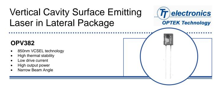
The OPV382 is a Vertical Cavity Surface Emitting Laser (VCSEL) packaged in a dome lens lateral package. VCSELs offer many advantages in sensing applications when compared to infrared LEDs. These devices require substantially lower drive currents to obtain the same amount of output power as LEDs. This feature allows VCSELs to be used in low power consumption applications such as battery operated equipment.
