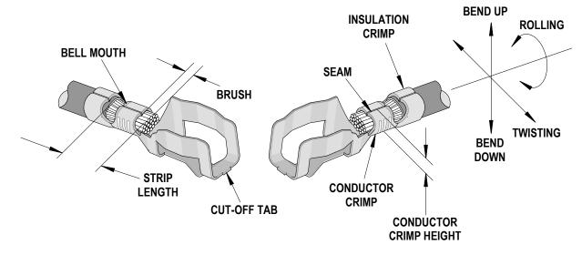
This illustration is a generic terminal representation and not an exact image of any terminal listed in the scope.
