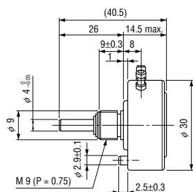
Unless otherwise specified, tolerance: ± 0.5 (Unit: mm)
