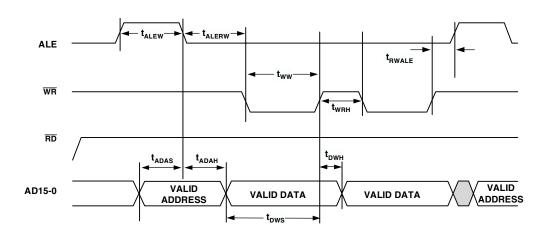
NOTE: FOR 16-BIT MEMORY WRITES, WHEN EMPP  $\neq$  0, ONLY ONE  $\overline{\text{WR}}$  PULSE OCCURS BETWEEN ALE CYCLES. WHEN EMPP = 0, MULTIPLE  $\overline{\text{WR}}$  PULSES OCCUR BETWEEN ALE CYCLES. FOR COMPLETE INFORMATION, SEE THE ADSP-2136X SHARC PROCESSOR HARDWARE REFERENCE.
