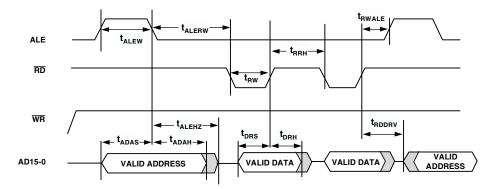
NOTE: FOR 16-BIT MEMORY READS, WHEN EMPP  $\neq$  0, ONLY ONE  $\overline{RD}$  PULSE OCCURS BETWEEN ALE CYCLES. WHEN EMPP = 0, MULTIPLE  $\overline{RD}$  PULSES OCCUR BETWEEN ALE CYCLES. FOR COMPLETE INFORMATION, SEE THE ADSP-2136X SHARC PROCESSOR HARDWARE REFERENCE.
