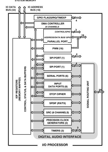
Figure 3. ADSP-21365/ADSP-21366 I/O Processor and Peripherals Block Diagram
