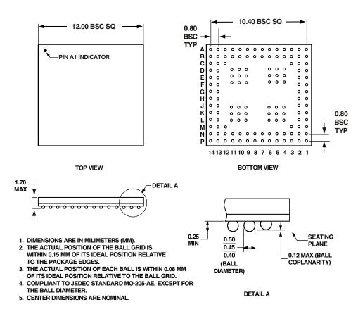
Figure 43. 136-Ball Mini-BGA (BC-136-2)
