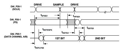
NOTE: SERIAL PORT SIGNALS (SCLK, FS, DATA CHANNEL A/B) ARE ROUTED TO THE DAI\_P20-1 PINS USING THE SRU. THE TIMING SPECIFICATIONS PROVIDED HERE ARE VALID AT THE DAI\_P20-1 PINS.
