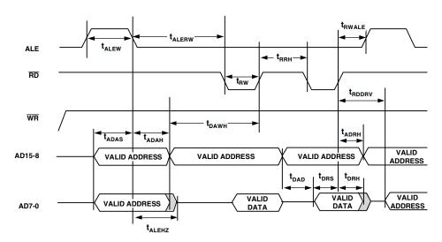
NOTE: MEMORY READS ALWAYS OCCUR IN GROUPS OF FOUR BETWEEN ALE CYCLES. THIS FIGURE ONLY SHOWS TWO MEMORY READS IN ORDER TO PROVIDE THE NECESSARY TIMING INFORMATION.
