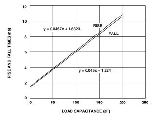
Figure 39. Typical Output Rise/Fall Time (20%–80%, V<sub>DDEXT</sub> = Max)
