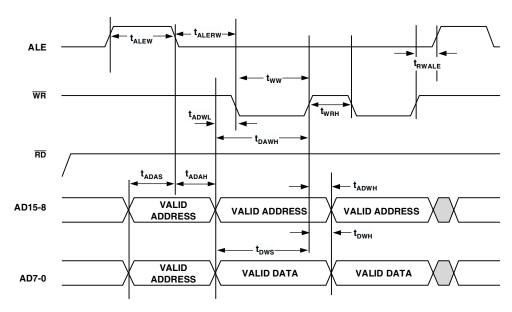
NOTE: MEMORY WRITES ALWAYS OCCUR IN GROUPS OF FOUR BETWEEN ALE CYCLES. THIS FIGURE ONLY SHOWS TWO MEMORY WRITES IN ORDER TO PROVIDE THE NECESSARY TIMING INFORMATION.
