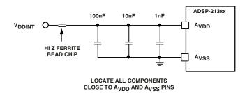
Figure 4. Analog Power (A<sub>VDD</sub>) Filter Circuit
