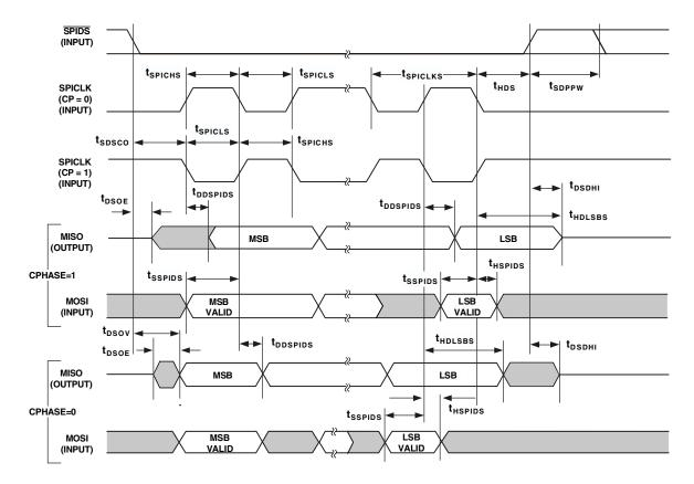
Figure 34. SPI Slave Timing
