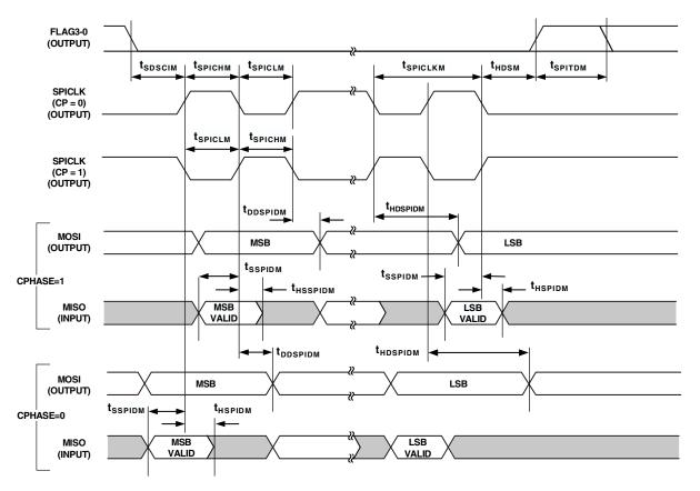
Figure 33. SPI Master Timing
