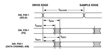
Figure 32. SPDIF Receiver Internal Digital PLL Mode Timing
