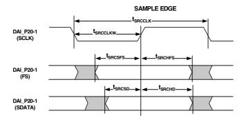
Figure 26. SRC Serial Input Port Timing
