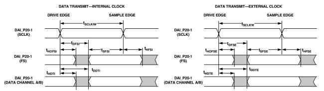
NOTE: EITHER THE RISING EDGE OR FALLING EDGE OF SCLK (EXTERNAL), SCLK (INTERNAL) CAN BE USED AS THE ACTIVE SAMPLING EDGE.
