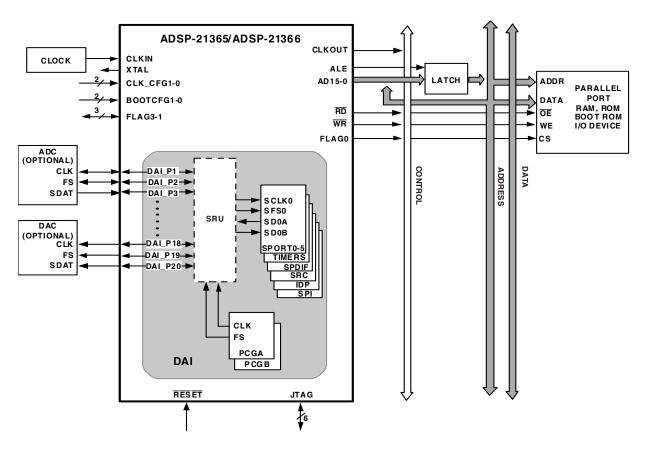
Figure 2. ADSP-21365/ADSP-21366 System Sample Configuration
