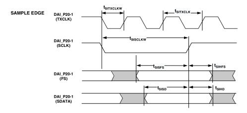
Figure 31. SPDIF Transmitter Input Timing
