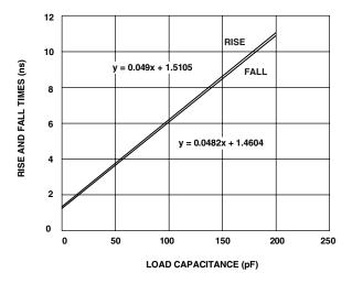
Figure 40. Typical Output Rise/Fall Time (20%–80%,  $V_{DDEXT} = Min$ )
