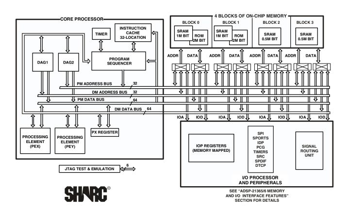
Figure 1. Functional Block Diagram—Processor Core
