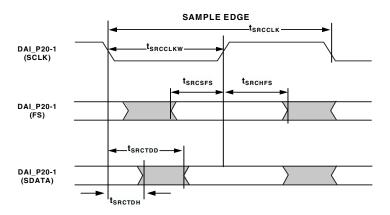
Figure 27. SRC Serial Output Port Timing
