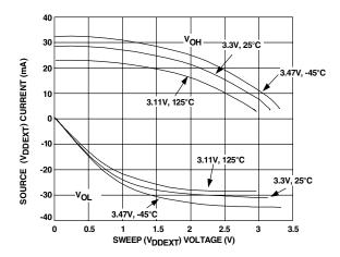
Figure 36. ADSP-21365/ADSP-21366 Typical Drive
