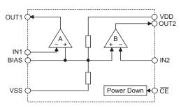
Output power to an  $8\Omega$  load with less than 10% (THD+N) from a 5V power supply. The very low standby current in shutdown mode contributes to the reduction of power consumption of battery-powered equipments. It provides 8-SOP package.
