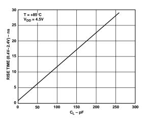
Figure 9. Typical Output Rise Time vs. Load Capacitance,  $C_L$  (at Maximum Ambient Operating Temperature)
