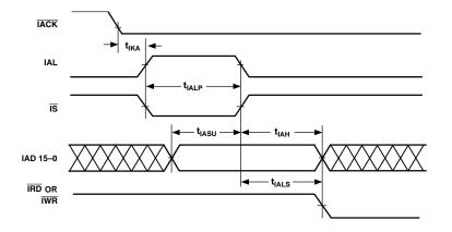
Figure 20. IDMA Address Latch
