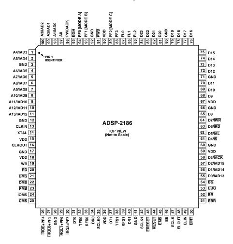
The ADSP-2186 package pinout is shown in the table below. Pin names in bold text replace the plain text named functions when Mode C = 1. A + sign separates two functions when either function can be active for either major I/O mode. Signals enclosed in brackets [] are state bits latched from the value of the pin at the deassertion of RESET.
