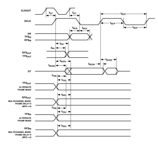
Figure 19. Serial Ports
