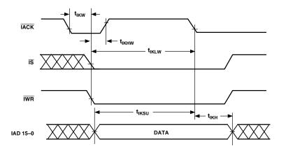
Figure 22. IDMA Write, Long Write Cycle
