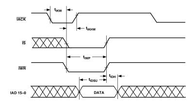
Figure 21. IDMA Write, Short Write Cycle
