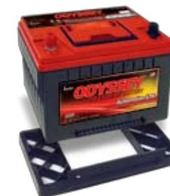
**OPTIONAL HEIGHT ADAPTOR** May be used on all 34-PC1500 models for installations where a group 24 or group 27 is required. Snap the adapter securely into place on the bottom of the battery. In some installations, the 34-PC1500 model with this adaptor may be used to replace a group 24F or 27F depending on required cable length.
