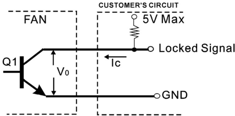
\*Transistor Q1 at "ON" position
