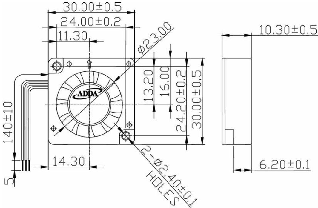
LEAD WIRES : UL 1571, AWG28, L = 140 +/- 10 mm
